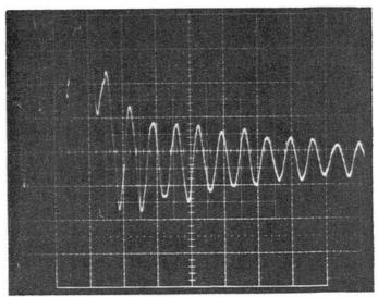
Fig. 2. Hydrophone response inside 6-cm diameter spherical brain model which was irradiated with a burst of three microwave pulses (10 μs) at a 24-kHz rate. Vertical scale was 100 μV/div; horizontal scale was 50 μs/div.
